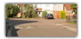
Speed tables are a raised section of road over a junction, with a ramp on each arm of the junction. The ramps are painted with white arrows to make them more obvious to motor vehicle drivers. The aim of the speed table is to slow motor vehicle traffic to a safe speed, as the ramps become uncomfortable for
