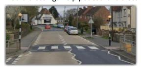
They have white strips painted onto the road in the crossing area, with flashing amber lights at both sides of the road on black and white striped poles. The curbs are dropped at both ends of the crossing. Traffic calming has its origins in the Dutch "Woonerf" schemes of the 1970's, and since then
